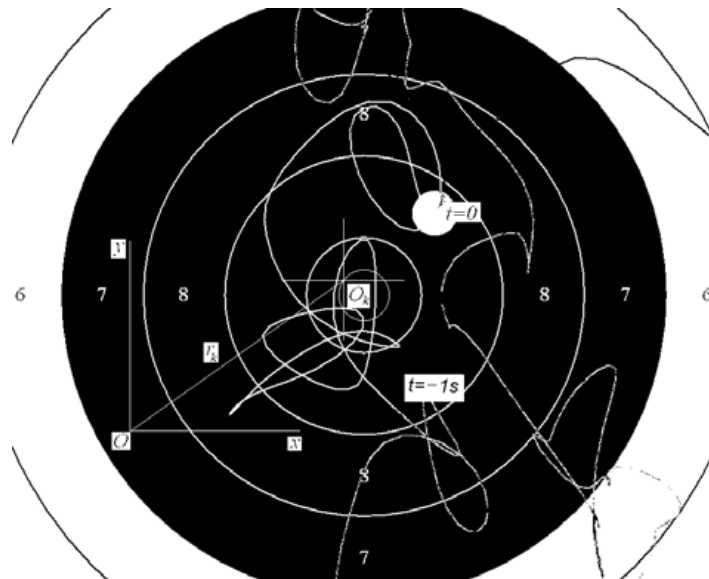
Fig. 1. Example of the target, showing parameters of the aim: t=-1 s is a beginning of the aiming trajectory, 1 s before pulling the trigger; t=0 – moment of the shot; O_K – trajectory of one shot's center; O – total average point of all aim's trajectories (60 shots)
