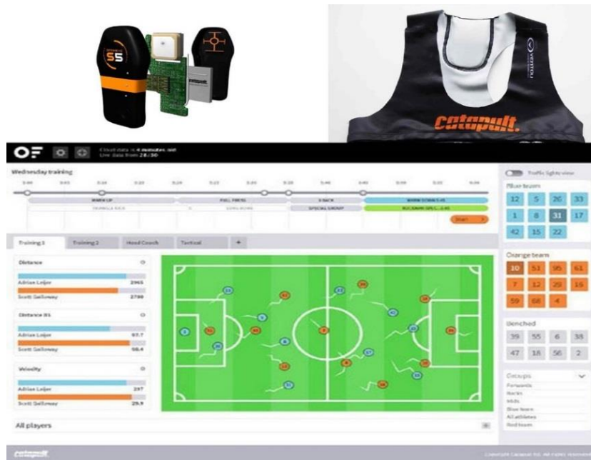
Fig. 1. Portable case with GPS-devices, elastic jacket, cloud-based analytic platform OpenField (Optimeye S5; Catapult Innovations of Australia, Melbourne)
